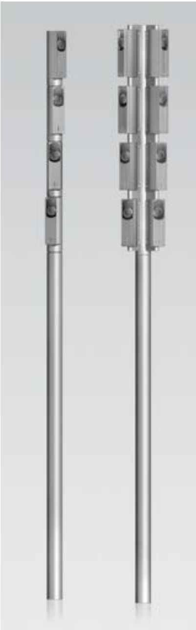
↗ HIT 7000 FP „folded pole“, stack mounting, bolt M24 connected ↗↗ HIT 7000 FR „folded regular“, fixed with mounting bracket vertically to the pole
